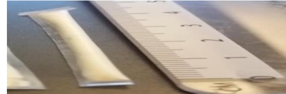
Full-scale TAF-TFPD prototype device 4 cm long x 2-2.5mm diameter
